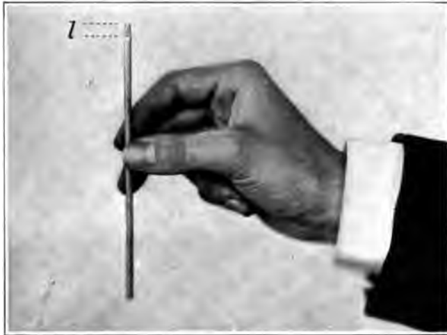
FIG. 36. Small organ pipe giving 15,600 vibrations per second.
